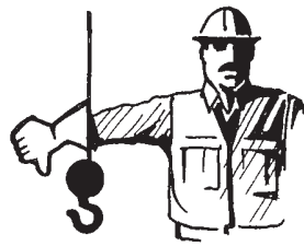
LOWER BOOM - Arm extended, fingers closed, thumb pointed downward.
