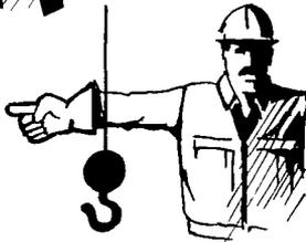
**SWING** - Arm extended, point with finger in direction of swing and boom.
