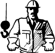
**RETRACT BOOM** - (telescoping boom) Both fists in front of body with thumbs pointed toward each other.
