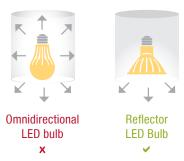
For down lights and recessed cans, install Energy Star® reflector LED bulbs. The light going upward from the omnidirectional bulbs can be wasted inside this fixture.
