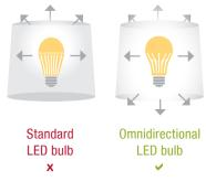
In table and floor lamps, you want the lights to shine in all directions, so look for Energy  $Star^{\circledast}\mbox{-labeled bulbs that}$  are omnidirectional.
